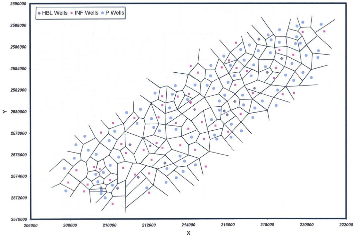
**Figure 2.** Location of 165 wells in the field. Well identified within colored drainage area are used as blind wells for validation of the analysis.
