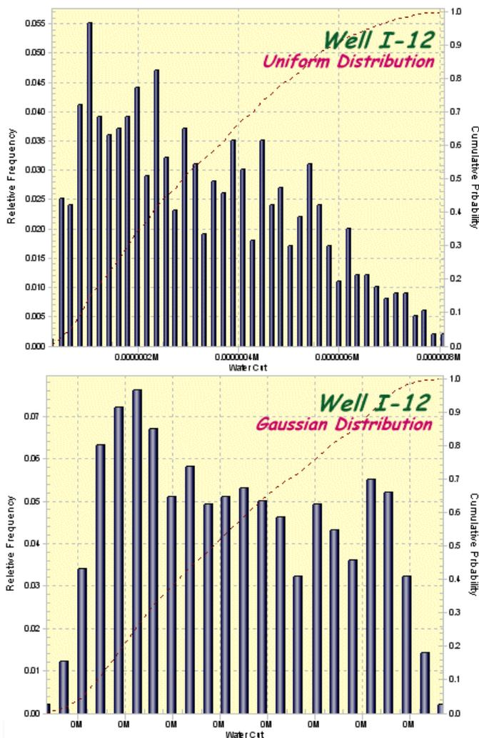
**Figure 8.** Probability distribution of instantaneous water cut (5<sup>th</sup> year) for well I-12 when uniform and Gaussian distribution is used for the top 5 KPIs.
