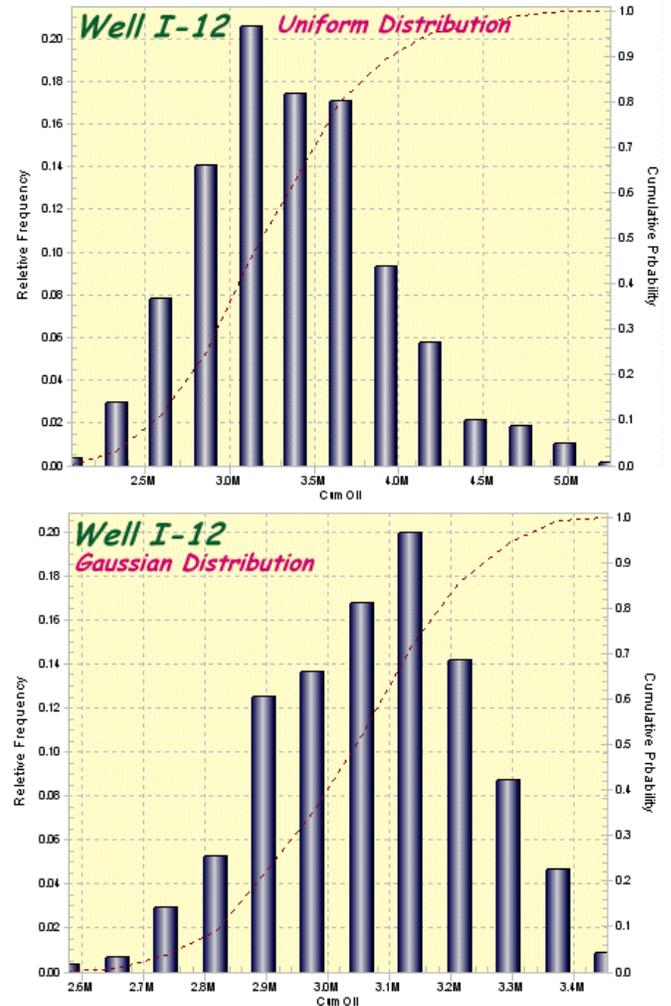
**Figure 6.** Probability distribution of cumulative oil production (5 years) for well I-12 when uniform and Gaussian distribution is used for the top 5 KPIs.
