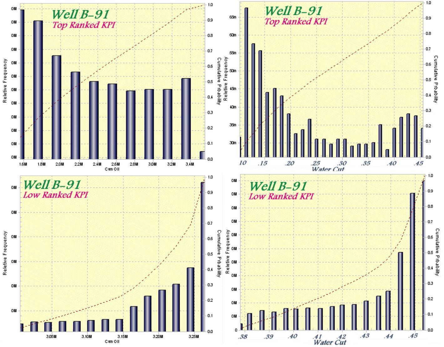
**Figure 9.** Probability distribution of instantaneous water cut (5<sup>th</sup> year) and 5 year cumulative oil production for well B-91. Monte Carlo Simulation performed analyzing uncertainties associated with two different reservoir parameters.
