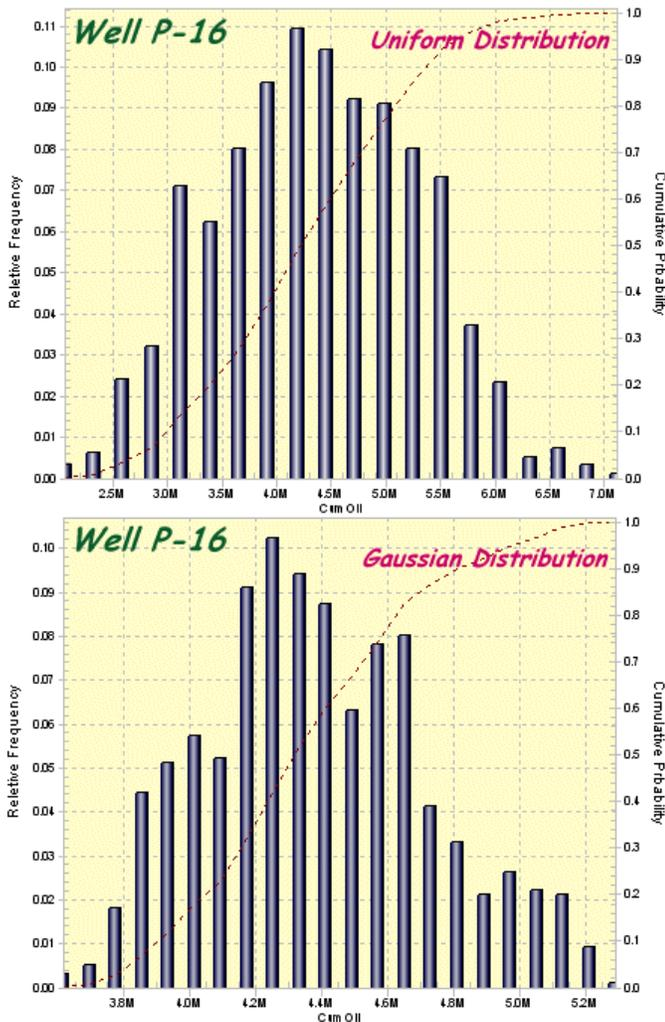
**Figure 5.** Probability distribution of cumulative oil production (5 years) for well P-16 when uniform and Gaussian distribution is used for the top 5 KPIs.
