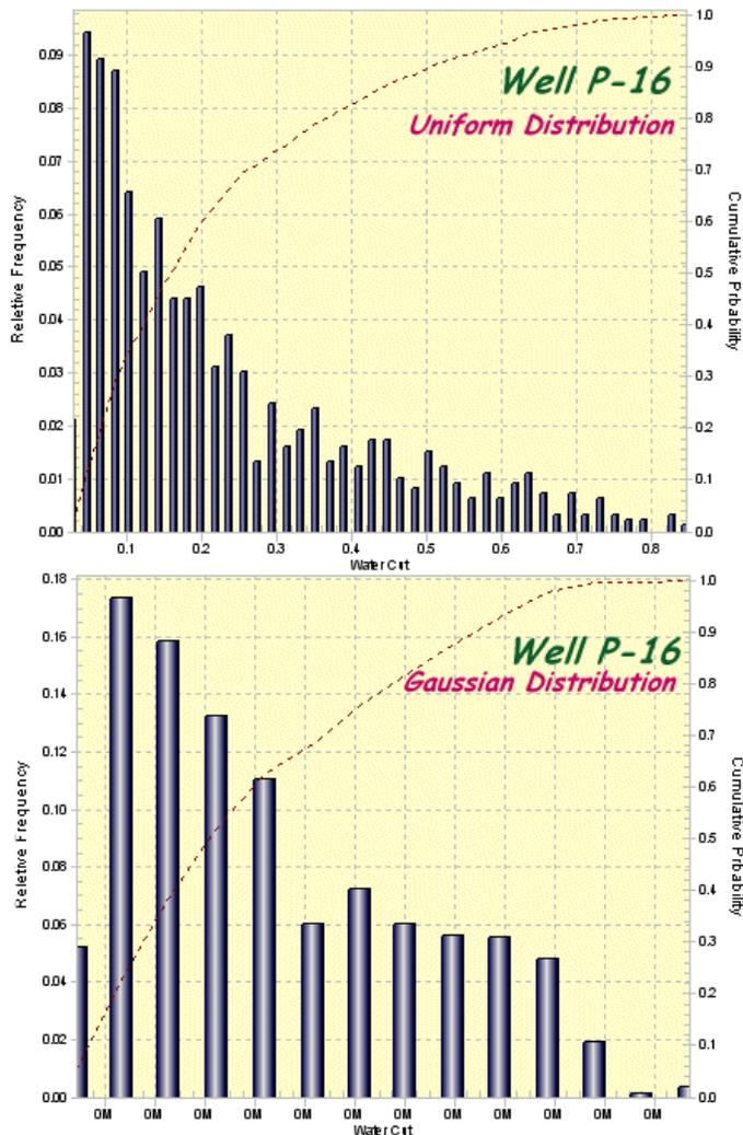
**Figure 7.** Probability distribution of instantaneous water cut (5<sup>th</sup> year) for well P-16 when uniform and Gaussian distribution is used for the top 5 KPIs.
